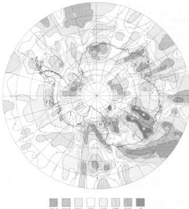
Fig. 3. MAGSAT total-field magnetic anomaly map over Antarctica. Units in gammas (nT). Capital letters indicate the approximate location of: A - Queen Maud Land, B - Enderby Land, C - Prince Charles Mountains, D - American Highlands, E - Gamburtsev Mountains, F - Wilkes Land, G - Transantarctic Mountains, H - Ross Embayment, I - Marie Byrd Land, J - Thurston Island, K - Ellsworth Mountains, L - Pensacola Mountains, M - Antarctic Peninsula.
