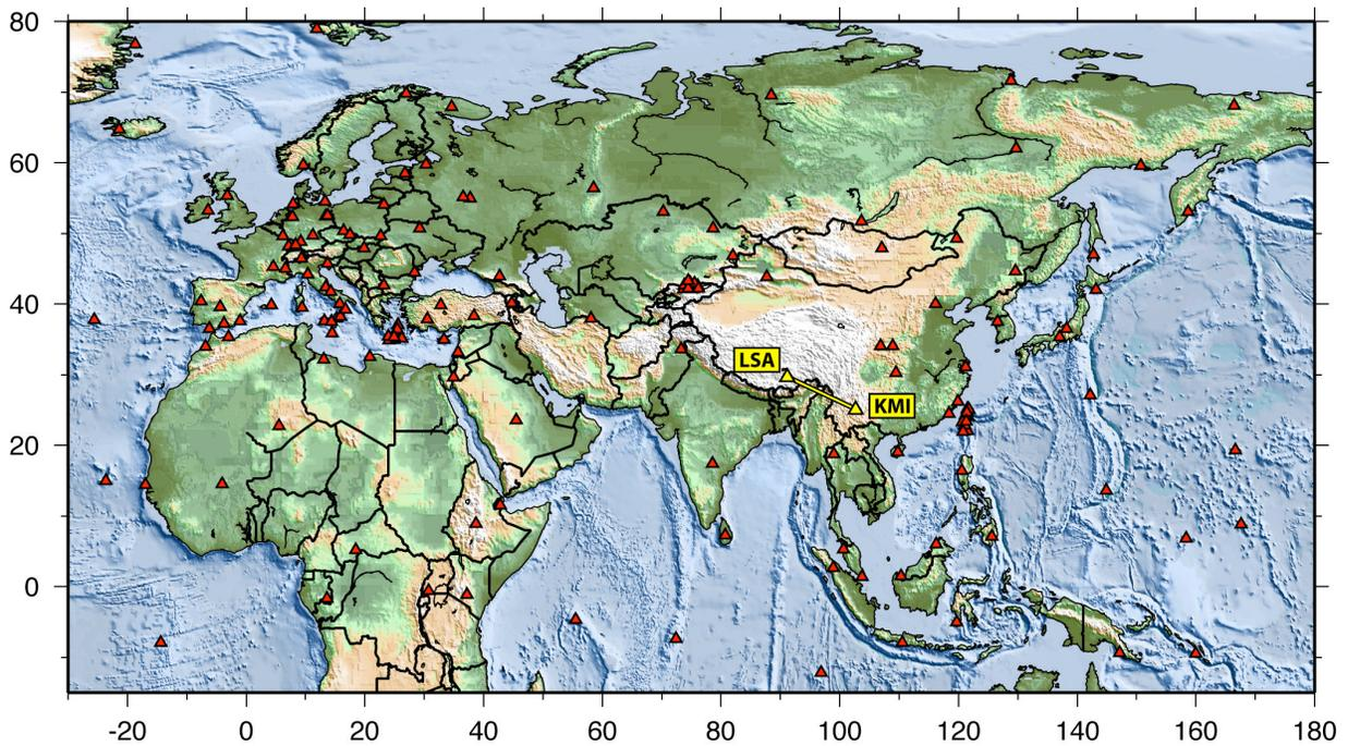
**Figure 5. Broad-band stations (red triangles) to be used for tomography across Eurasia and North Africa. The path between GSN stations LSA (Lhasa, Tibet) and KMI (Kunming, China) is highlighted, and corresponds to the cross-correlations shown in Figure 6.**
