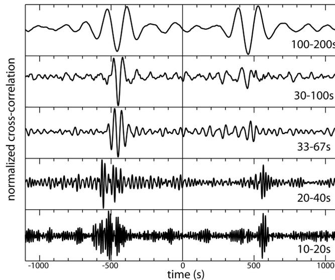
**Figure 3.** Broad-band cross-correlations between two North American GSN stations: CCM (Cathedral Cave, MO) and HRV (Harvard, MA). The cross-correlations are for 1 month of data from November, 2003. The time axis is the cross-correlation lag (in sec). In this case, positive lag corresponds to waves traveling from CCM to HRV and negative lag to waves from HRV to CCM. The pass band in each case is indicated.
