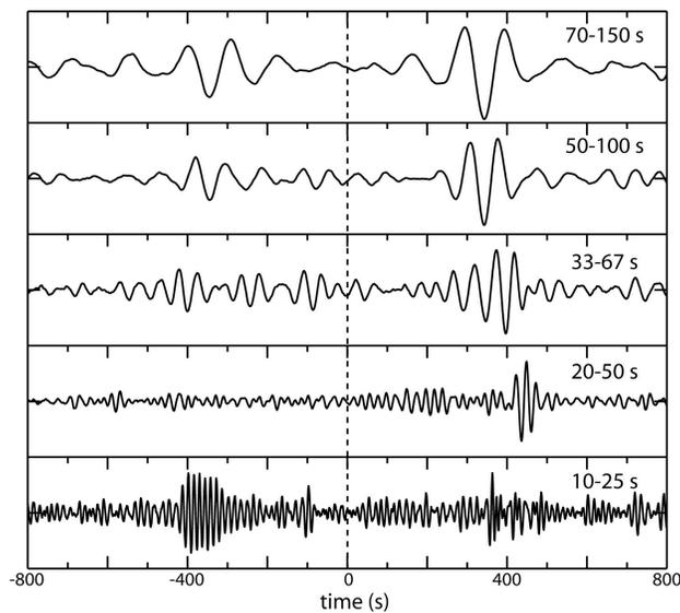
**Figure 6. Broad-band cross-correlations between two Asian GSN stations: LSA (Lhasa, Tibet) and KMI (Kunming, China). The cross-correlations are for 1 month of data from January, 2004. The time axis is the cross-correlation lag (in sec). In this case, positive lag corresponds to waves traveling from KMI to LSA and negative lag to waves from LSA to KMI. Each pass-band is indicated.**
