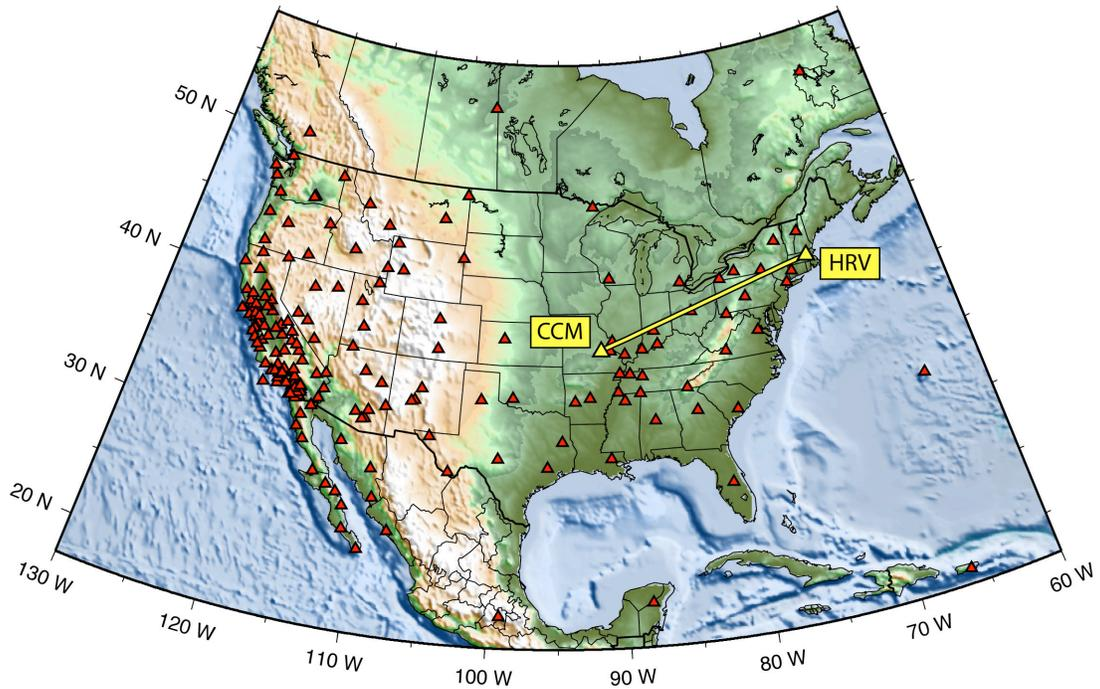
**Figure 2.** Current backbone network across the US. As a test-bed for continental scale tomography across Eurasia and North Africa, 125 broad-band stations (red triangles) are used within and surrounding the US. The path between GSN stations CCM (Cathedral Cave, MO) and HRV (Harvard, MA) is highlighted, and corresponds to the cross-correlations shown in Figure 3.
