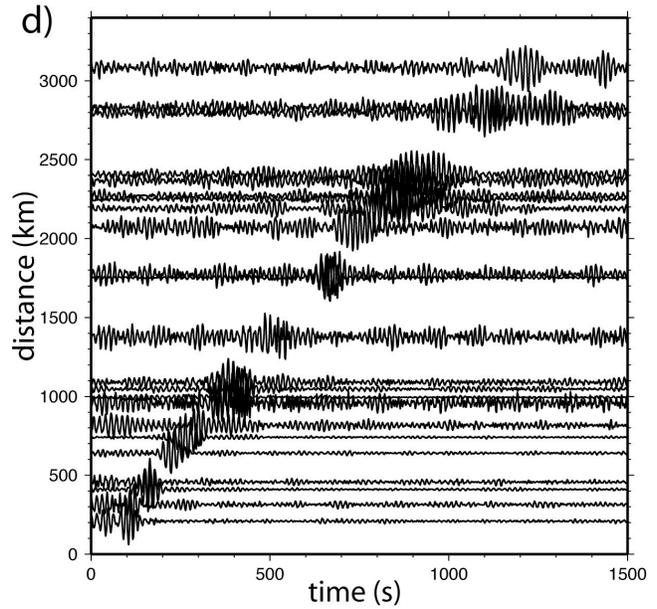
**Figure 7. Example receiver gathers (record sections for particular stations) for one-month cross-correlations (Jan. 2004) bandpassed between 10 and 20 sec period for two European stations: CSS (Cyprus) and IBBN (N. Germany). (a) Paths between stations linked to CSS. (b) Receiver gather for station CSS. (c) Paths between stations linked to IBBN. (d) Receiver gather for station IBBN. In (b) and (d) only positive cross-correlation lags are shown.**
